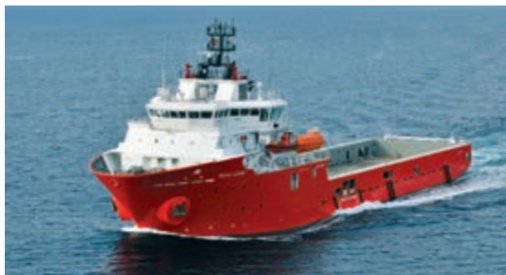
L-class vessels, introduced in 2014, are large fuel-efficient platform supply vessels well-suited to operating in deeper waters.
